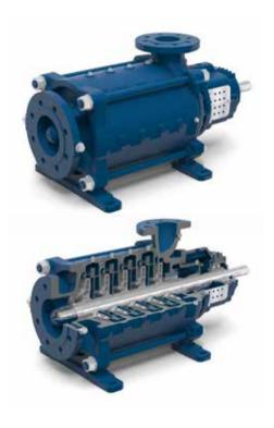
Special features: highest suction capability (the lowest NPSH) thanks to ideal axial inlet flow, reduced wear due to fewer parts, small horizontal footprint
