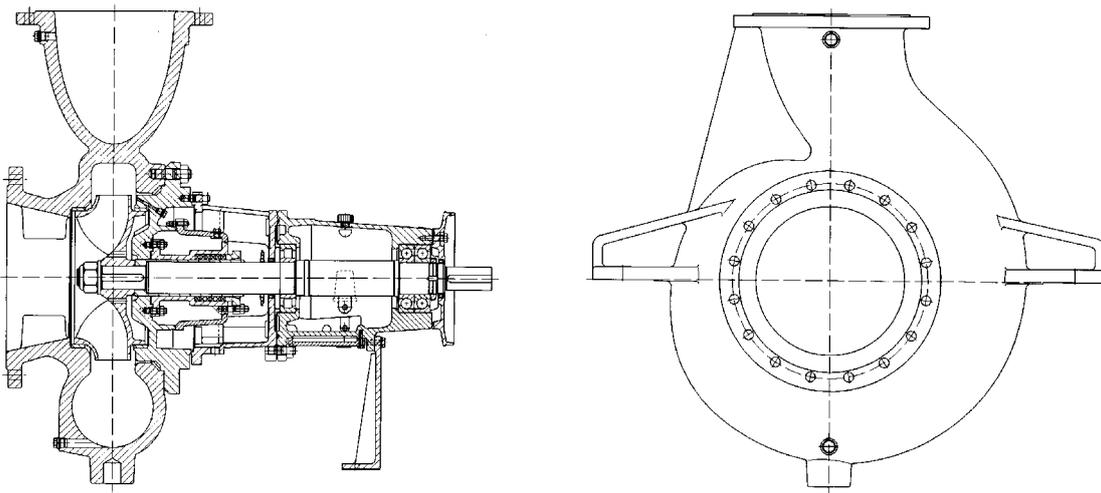
Due to the centerline casing feet and the additional support feet a negative influence is avoided on the coupling alignment caused by thermal expansion of the casing at high operating temperatures.
