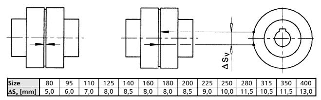
Attention If wear is heavy, it must be assumed that the motor is not properly aligned with the pump or that the distance between the coupling sections has changed.
